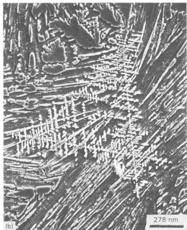
Figure 5 Scanning electron micrographs of the central region of a \text{Pd}_{77.5}\text{Au}_6\text{Si}_{16.5} droplet with diameter D = 1000 \mu\text{m} : (a) unbranched dendritic growth of \text{Pd}_3\text{Si} ; (b) branched triangular dendritic growth of \text{Pd}_3\text{Si} .
